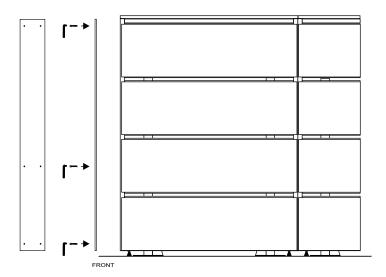
■ End-plate code 1022/136 or 1022/102 fixed to wall-unit with 6 bolts incl. nuts per end-plate.
