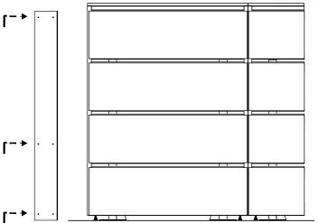
■ Corner section code 1020-90/136 or 1020-90/102 fixed to 2 wall-units with 12 bolts incl. nuts.
