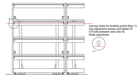
Use key-holes for levelling points (figur 1).
