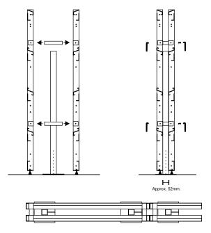
■ When fixing wall-unit use 4 pcs of sectional fittings L11cm. per each two-sidet wall-units. There must be a distance between the 2 wall-units of min.52mm. to fit the topplate fitting 1002/A, topplate 1102/A and the end-plate 1022/136 or 1022/102.
